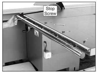
Figure 23. Attaching the scale.
